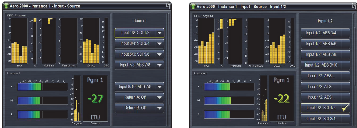
Figure 1-8 Left: inputs for a given instance; Right: available choices for AES or SDI pair
