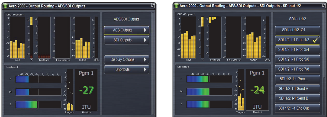
Figure 1-9 Left: main AES outputs (BNC and DB25) and SDI outputs; Right: SDI output setup
