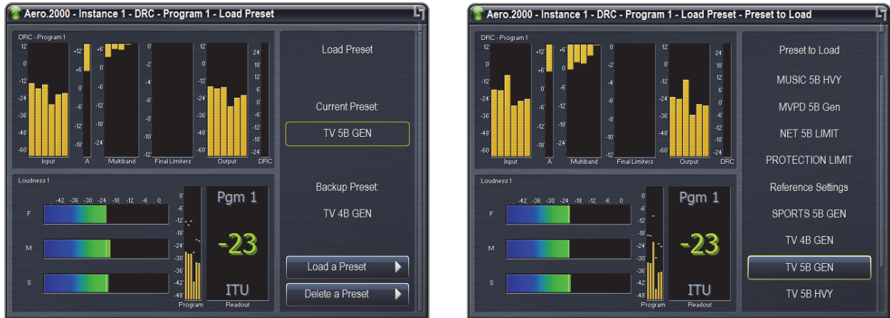
Figure 1-12 Left: current preset for Instance 1, Program 1; Right: partial list of available presets
